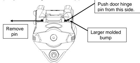
When enough of the door hinge pin becomes exposed it can be removed by grasping it with the pliers (slightly lift the pin upwards to clear the smaller molded bump) and sliding it free.
